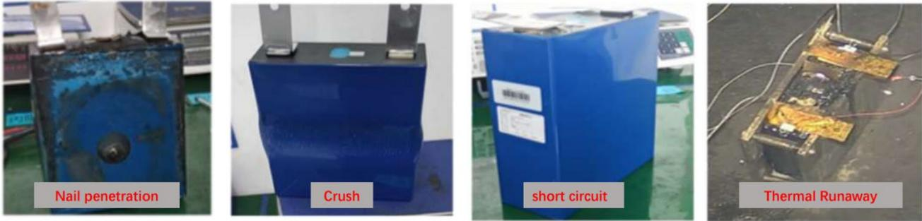
Figure 4-5 REPT's 280 Ah cells after different safety tests
