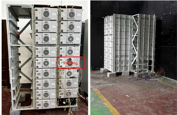
**Figure 5-2 Aero-C UL 9540A rack level test layout and set up**
