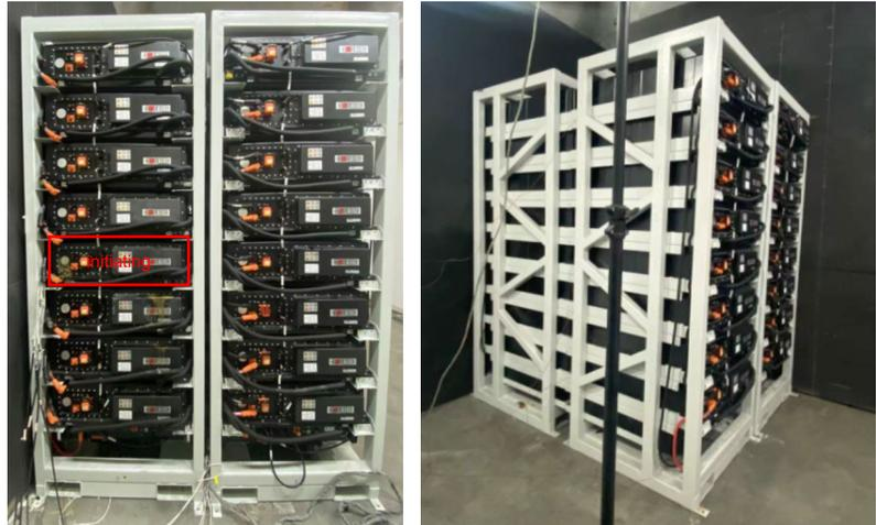
**Figure 5-3 Aqua-C UL 9540A rack level test layout and set up**
